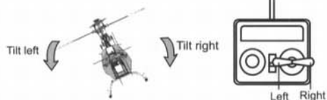
Flying control of Left/Right cyclic
